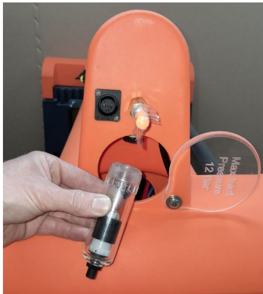
Figure 27. Air regulator filter bowl
