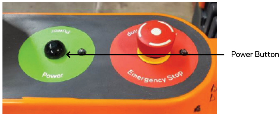
Figure 21. The Sheep Auto Drafter Power button.
