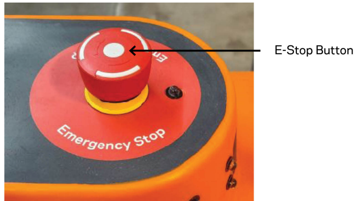
Figure 25. E-Stop button position.
