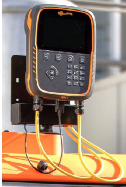
Figure 19. The 3 cables connected to the Weigh Scale indicator.
